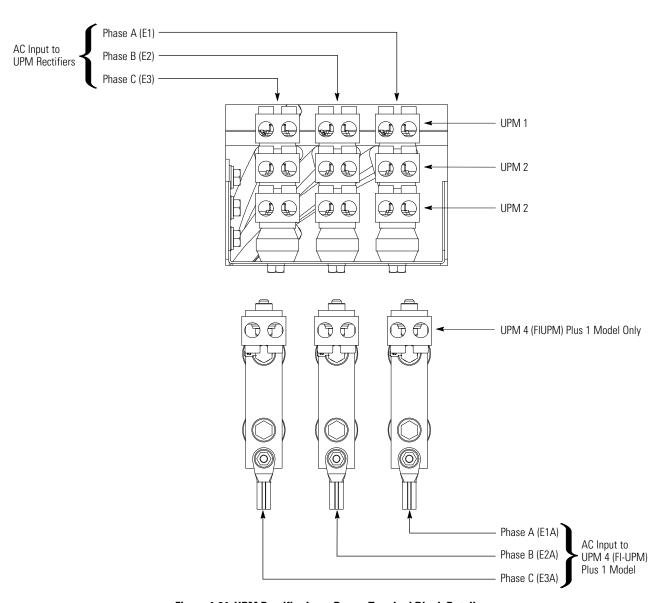
Figure 4-24. UPM Rectifier Input Power Terminal Block Detail
